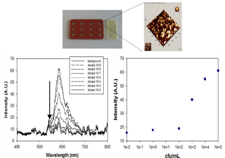
**Figure 5.** (Top) AFM image of SIFs as the substrate for the MAMEF assay. (Bottom) The fluorescence spectra of the fluorophore probe after incubation with target DNA. The intensity of the fluorophore probe is directly related to the varying
